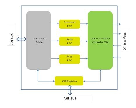
Caption: SmartDV's DDR5 and LPDDR5 Design IP (in green box) offer low power and latency, reduced gate count for increased memory interface bandwidth.
